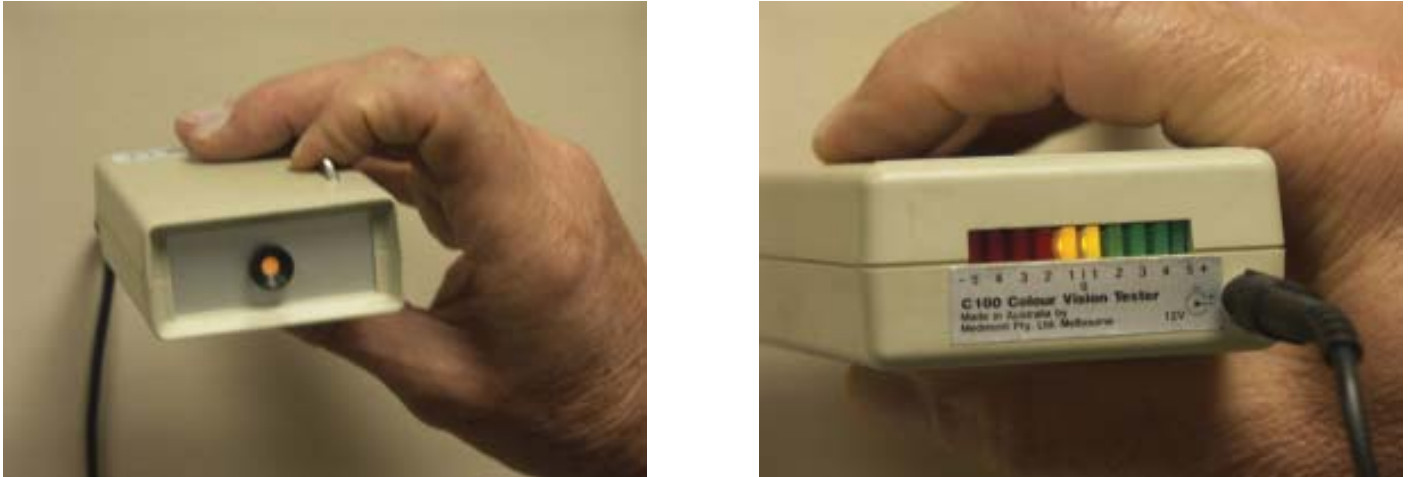
Figure 2. The Medmont C-100 test. Left. The subject views a yellowish flickering light generated by alternating red and green LEDs and adjusts the control knob until the flicker disappears or is a minimum. Right. The settings chosen to achieve no or minimum flicker are read on an arbitrary scale from -5 to +5 where +2.0 to -2.0 is the extreme range of normal settings but typically settings are within \pm 1.0 . The scale is colour-coded red for protan settings, green for deutan and yellow for normal. The colour-coded scale lights correspond to integers (1, 2, 3 ...) but can be interpolated to 0.5, when two adjoining lights are illuminated.
